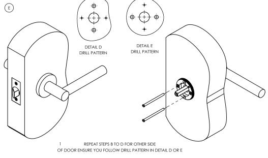
INSERT THROUGH BOLTS DURING STEP C
