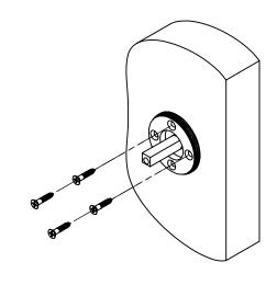
SECURE THREADED INNER DUMMY SPINDLE USING WOOD SCREWS SUPPLIED
