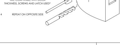
1 INSTALL LEVER AND ROSE ASSEMBLY AND SCREW IN NO.6 FIXING SCREWS SUPPLIED
