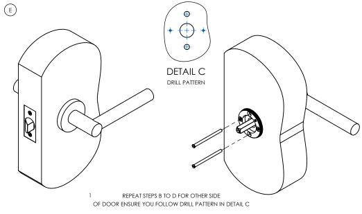
INSERT THROUGH BOLTS DURING STEP C
