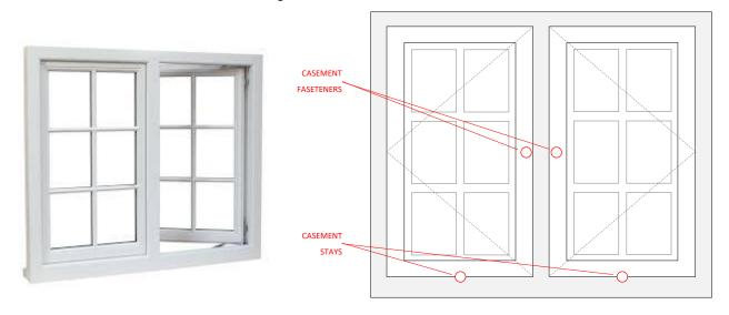
Older style timber casement windows are fitted with traditional ironmongery such as a casement stay and casement fastener as illustrated above. Modern casement windows may be manufactured with an integral friction stay and an espagnolette (multi-point) locking device which is operated by an espagnolette handle.
