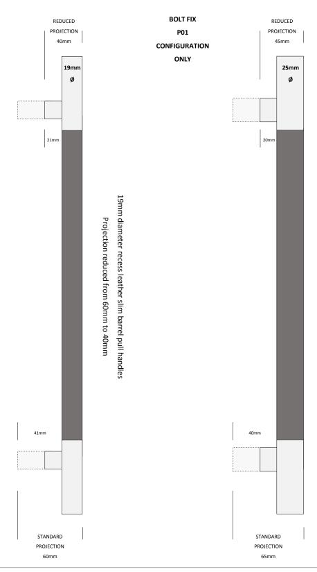
25mm diameter recess leather, recess amalfine, solid and solid hammered pull handles
